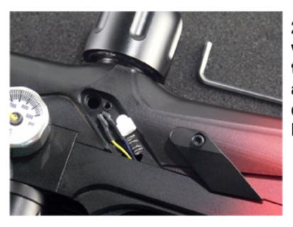
2. Clean the ball detent with water and dry thoroughly. Clean the area around the ball detent if needed. Do not lose the small spring.
