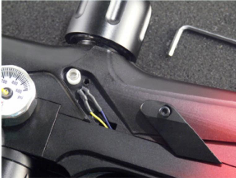
**1. Remove the eye cover by unscrewing the 4-40x1/4 SHCS.**
