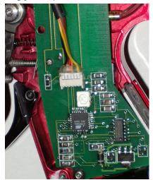
To access the programming port of your Chaos Alias board, you must remove the grip and clamshell half that covers the circuit board. The programming port is located directly over the LED.
