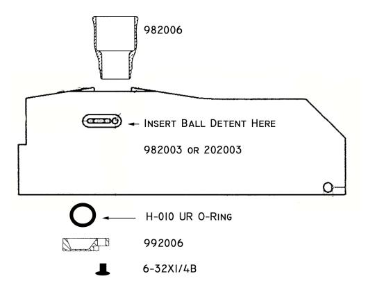
APPLY A SMALL DAB OF RED LOCTITE TO THE THREADS OF FEED TUBE 982006. CAREFULLY SCREW INTO UPPER RECEIVER. TIGHTEN FIRMLY, WITHOUT PUTTING UNBALANCED STRESS ON THE FEED TUBE, WHICH MAY CAUSE IT TO BEND. WIPE OFF ANY EXCESS LOCTITE.
