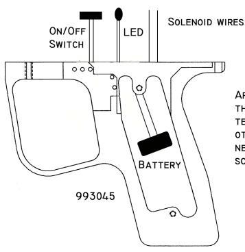
ARRANGE THE WIRING HARNESS WIRES SO THAT THE BATTERY CONNECTION AND BOARD TERMINAL REST INSIDE THE GRIP AND ALL OTHERS FACE UP OUTSIDE THE GRIP. IF NECESSARY, THREAD THE ON/OFF SWITCH SCREW HOLES WITH A 3-48 TAP.
