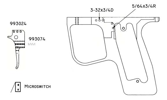
PLACE TRIGGER SPRING 993074 IN MIDDLE HOLE OF TRIGGER 993024 HOLES, IN THE BACK BEHIND THE SCREW. SLIDE TRIGGER INTO GRIP FRAME 993045. LINE UP HOLES ON TOP OF TRIGGER 993024 WITH HOLES ON TOP OF GRIP FRAME 993045. SCREW TWO 8-32XI/4 SET SCREWS INTO THREADED HOLES ON TOP SIDE OF TRIGGER FRAME THREE HOLES, SO THAT THEY HOLD THE DOWEL PIN IN PLACE. USING A GUIDE PIN, HOLD MIDDLE HOLES IN ALIGNMENT. PRESS 3-32X3/4 DOWEL PIN INTO CENTER HOLE OF GRIP FRAME 993045, AND THROUGH TRIGGER HOLE.
