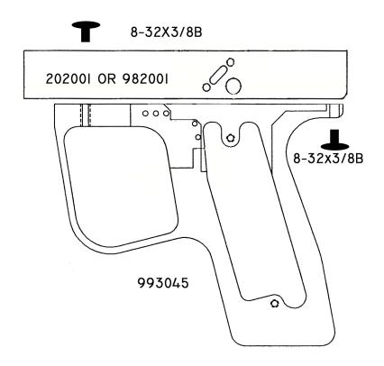
PULL THE WIRES THROUGH THE CENTER OF THE TRAY 982001 OR 202001 AND THEN SCREW THE TRAY TO THE GRIP FRAME 993045 WITH TWO 8-32x3/8 BUTTONHEAD SCREWS. MAKE SURE SCREWS ARE TIGHT. THEN INSTALL THE LED INTO THE TRAY BY PUTTING THE BLACK COVER ON THE OUTSIDE AND PUSHING THE LED THROUGH THE BACK TO BE PINNED BY THE BLACK COVER. USING TWO 3-48X3/16 PAN HEAD PHILLIPS MACHINE SCREWS, INSTALL THE ON/OFF SWITCH. LEAVE THE SOLENOID LAYING IN THE TRAY UNTIL TIME TO SCREW IT TO THE MANIFOLD.
