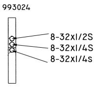
APPLY A SMALL DAB OF BLUE LOCTITIE TO EACH SCREW. SCREW THE 8-32XI/2 SET SCREW IN FROM FRONT UNTIL IT JUST BARELY POKES OUT THE BACK. SCREW THE MIDDLE 8-32XI/4 SET SCREW IN FROM THE FRONT UNTIL FLUSH. SCREW THE BOTTOM 8-32XI/4 SET SCREW IN UNTIL ABOUT FLUSH IN THE BACK OF THE TRIGGER 993024.
